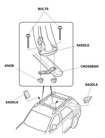
Position the two hydro-glide assemblies on the rear crossbar. Loosely install the hydro-glide assemblies using one bracket, two bolts, and two knobs for each assembly. The distance between the two assemblies should be the same width as the kayak.
