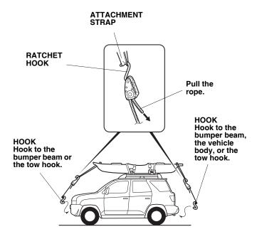
13. To loosen the rope, push up on the ratchet strap lever, then pull on the other end of the rope.
