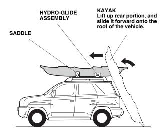
4. Adjust the distance of the saddles and hydroglide assemblies to the same width as the kayak, then secure the saddle and the hydro-glide assemblies by tightening the knobs you installed in steps 1 and 2.
